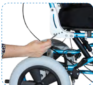
SEAT/BACK MECHANICAL RECLINING WITH QUICK RELEASE PIN
